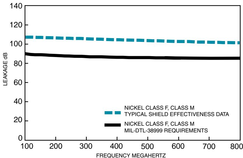
Amphenol® Tri-Start connectors provide EMI/EMP shielding capability which exceeds MIL-DTL-38999 Series III requirements.
