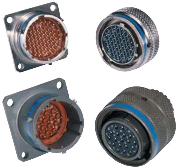
**Amphenol® LJT and JT Series subminiature cylindrical connectors are qualified to MIL-DTL-38999\*, Series I and II respectively. These connectors were developed to meet the needs of the aerospace industries, and provided the impetus for development of the MIL-C-38999 specifications, which recently were superseded by MIL-DTL-38999. Meeting or exceeding MIL-DTL-38999 requirements, Amphenol® JT/LJT connectors feature:**
