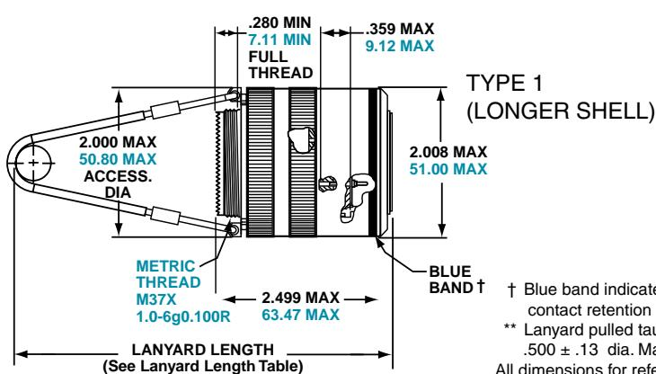
† Blue band indicates rear release contact retention system
