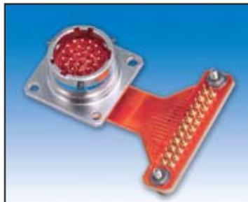
**Flex Circuity for Attachment to Printed Circuit Boards**
