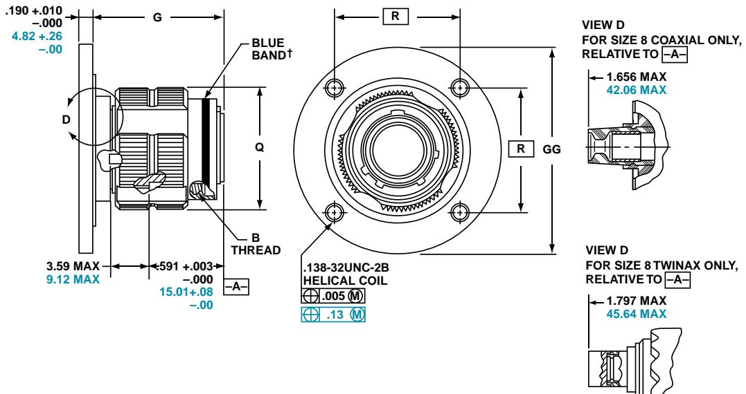
† Blue band indicates rear release contact retention system
