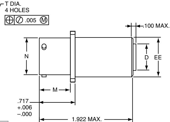
Plug movement required to clear FSJT receptacles: .625 min.
