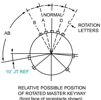
A plug with a given rotation letter will mate with a receptacle with the same rotation letter. The AB angle for a given connector is the same whether it contains pins or sockets. Only the master key/keyway rotates in the shell, and the insert always remains in the same position relative to the minor keys.
