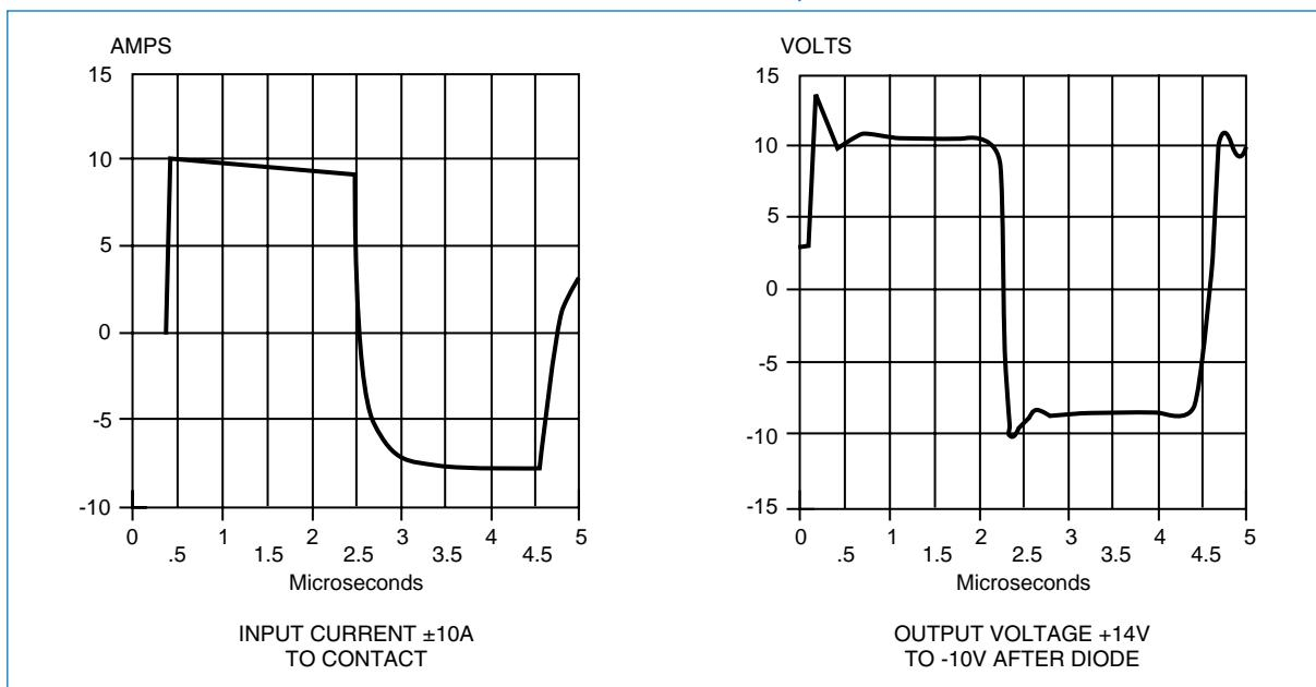
The Amphenol® Energy Shunting Assembly (ESA) is a simple, compact unit which provides lightning and electromagnetic pulse (EMP) protection of systems in which many signal lines enter sensitive electronic equipment. The efficient packaging of the ESA circumvents the concept of one protective device per line. It provides a surge arrestor which has the advantage of space saving and simplified assembly when compared to current protective devices which range from diodes to large spark gaps.
