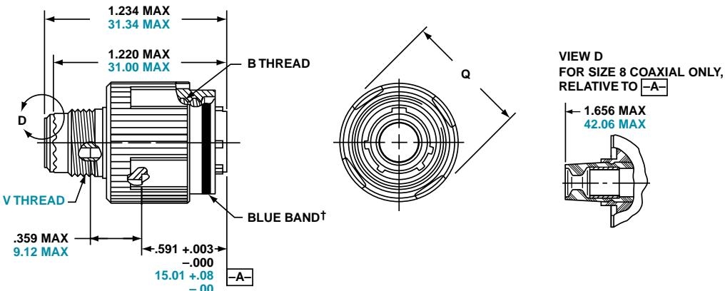
† Blue band indicates rear release contact retention system
